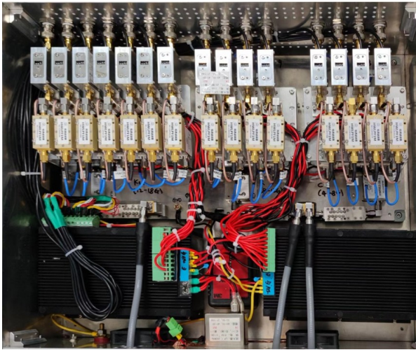
Figure 7. Photograph of the integrated X-, C- and Ku-band subsystems.
