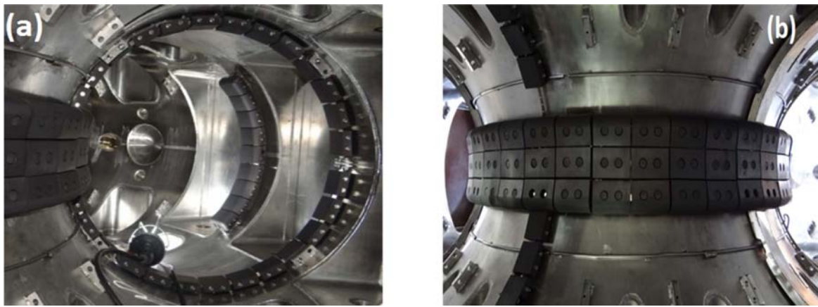
Figure 4. (a) Safety and poloidal ring limiters. (b) Toroidal belt limiter.
