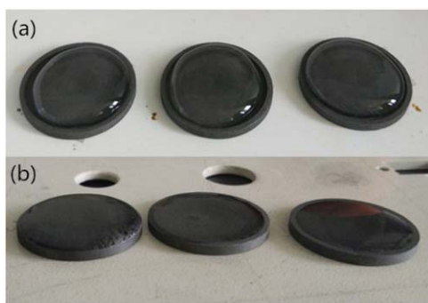
Figure 5. The difference between the water on hydrophobic and hydrophilic graphite flakes.
