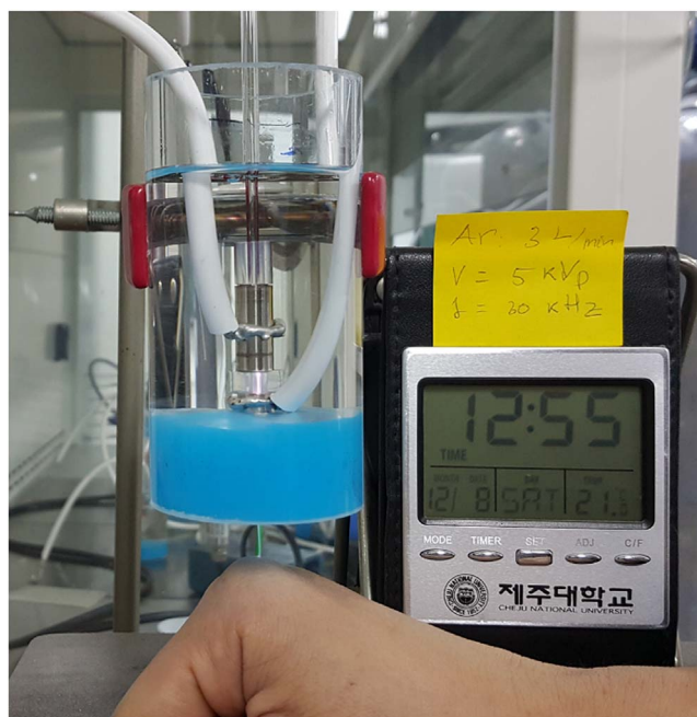
Figure 7. The Ar plasma jet interaction with human skin (applied voltage: 5 kV; frequency: 30 kHz; Ar flow rate: 3 slm).
