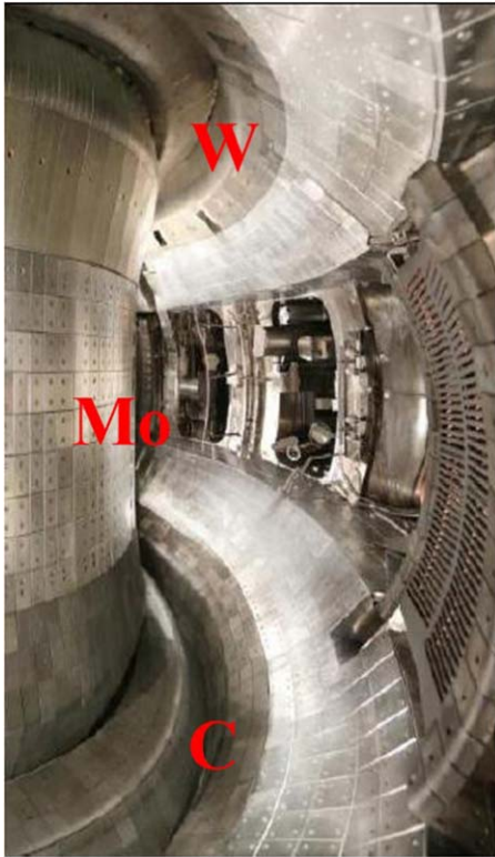
Figure 1. Internal view of EAST vacuum vessel with different PFMs: upper tungsten divertor, lower carbon divertor and first wall molybdenum tiles.
